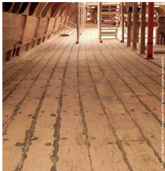
Douglas fir lumber from French forests was used in the reconstruction of the Hermione naval ship (a replica of the frigate used by Lafayette).
