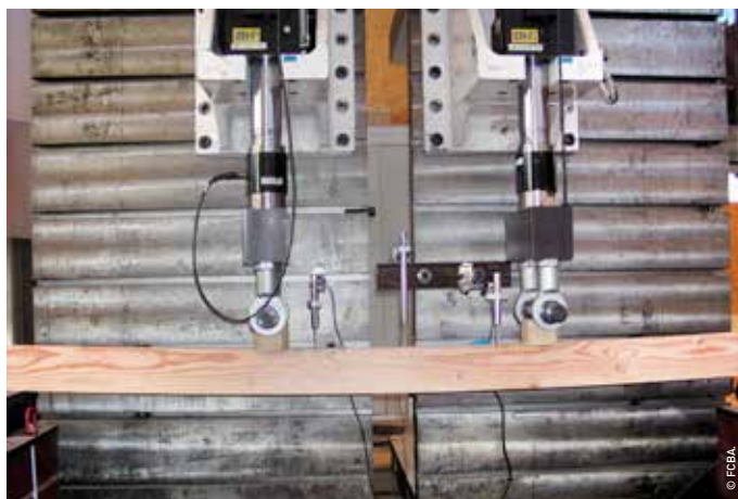
Mechanical strength test on Douglas fir lumber.
